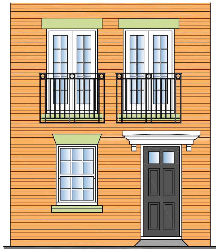
TYPICAL ELEVATION WITH JULIET BALCONY
