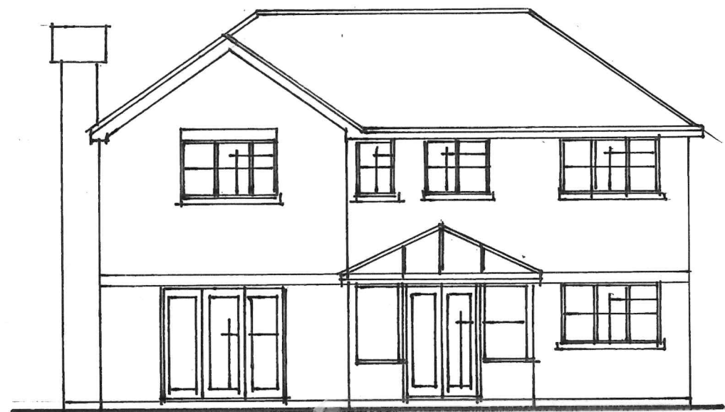
REAR ELEVATION - EXISTING
