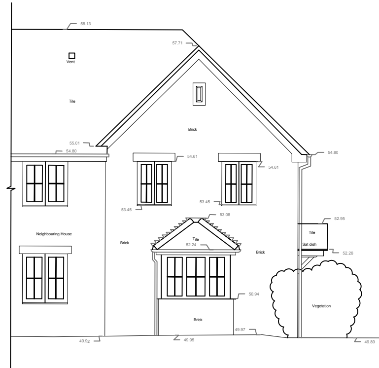
2 Existing Side Elevation - North West Scale: 1:100 @ A3
