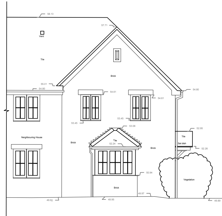
2 Existing Side Elevation - North West Scale: 1:100 @ A3
