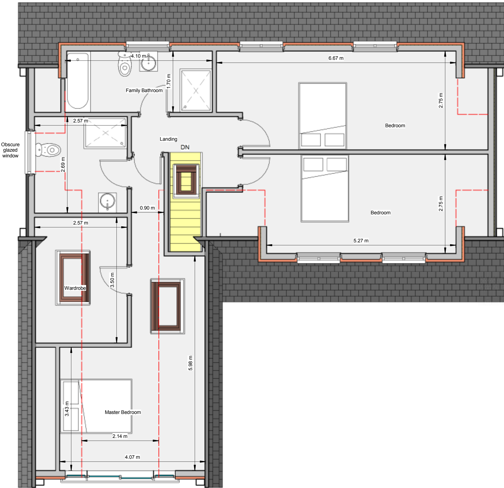
6 Proposed First Floor Plan 1 : 50
