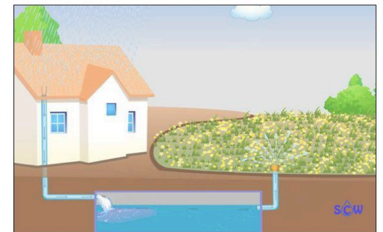
Rainwater Harvesting Example
