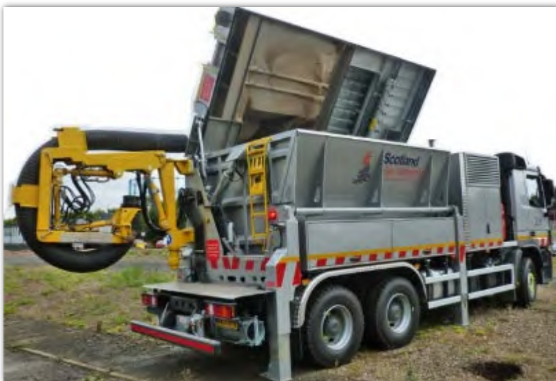
Figure 17. Large Vacuum Excavator
