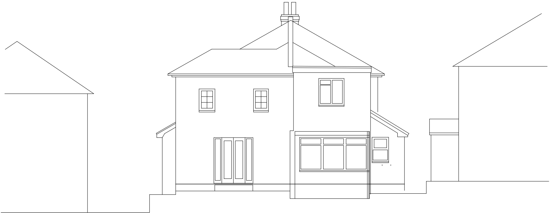
7.00m DATUM EXISTING NORTH ELEVATION 1:100
