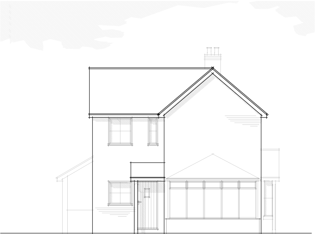
EXISTING SIDE ELEVATION (facing due south) SCALE 1:100
