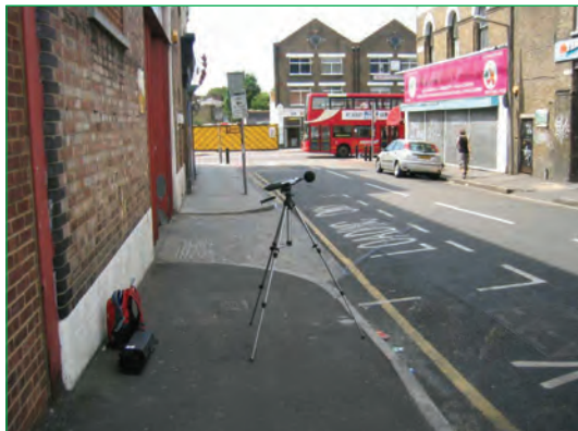
Figure 4.34 Façade noise monitoring equipment (courtesy Arup)
