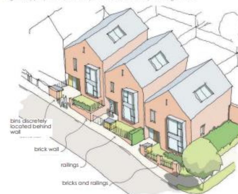
Fig.32: Appropriate boundary structures for front private gardens
