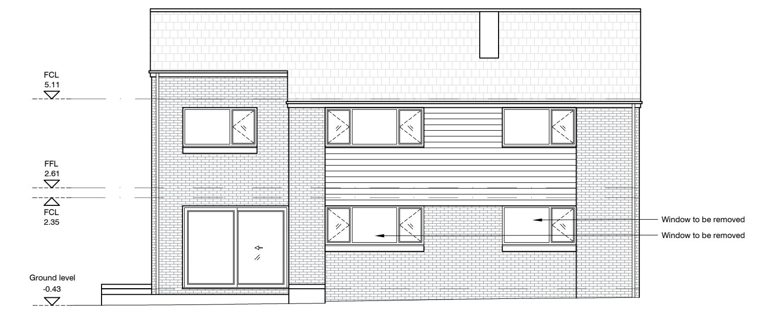
5 SIDE (SOUTH EAST) ELEVATION 1:100
