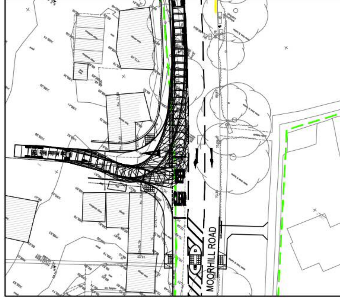
ARTICULATED VEHICLE TURNING LEFT OUT OF SITE IN FORWARDS GEAR.
