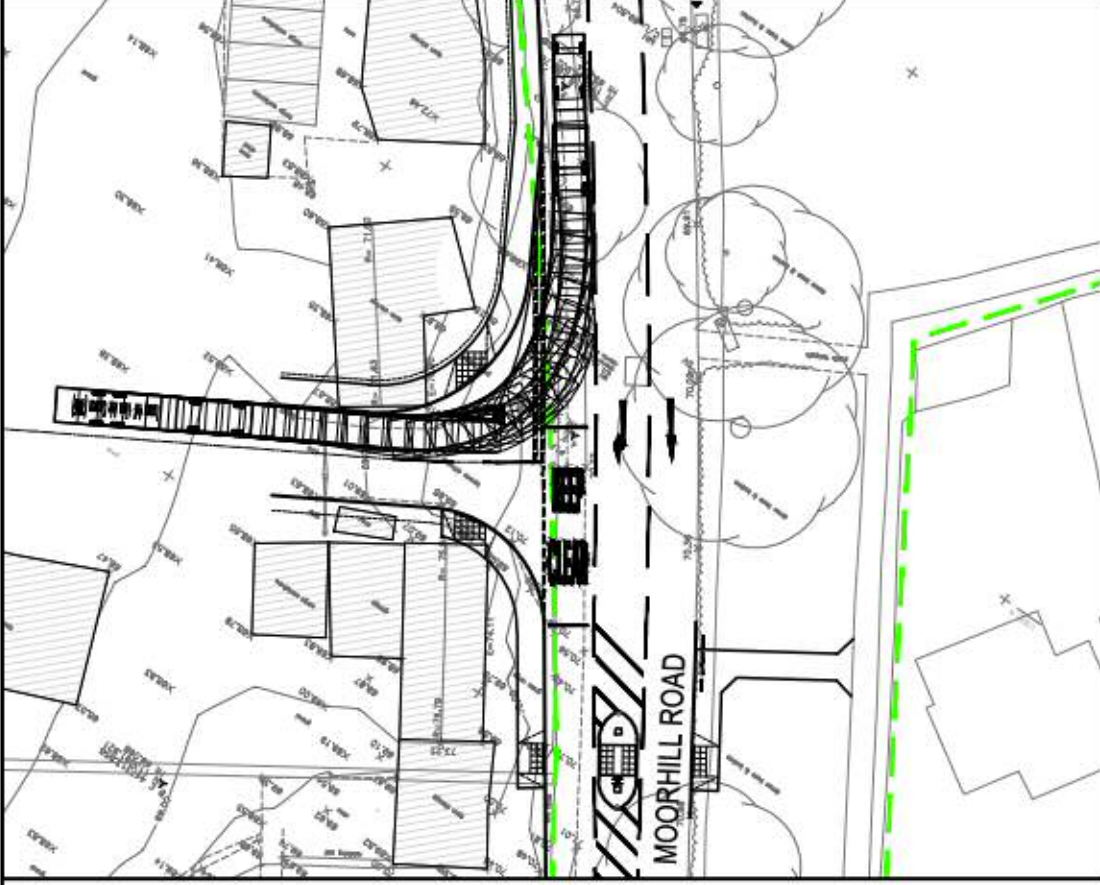
TWIN AXLE CARAVAN TURNING LEFT OUT OF SITE IN FORWARDS GEAR.
