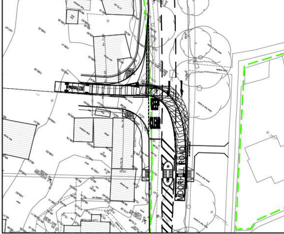
PANTECH TURNING RIGHT OUT OF THE SITE ACROSS THE GHOST ISLAND AND TURNING LANE IN FORWARDS GEAR.
