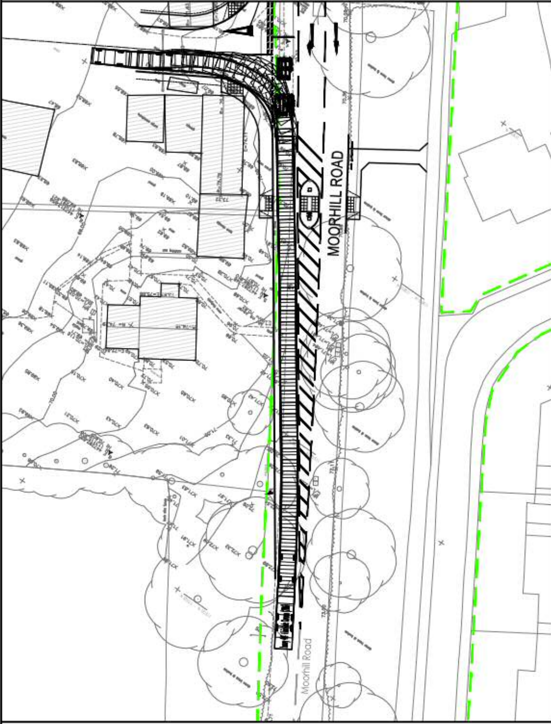
TWIN AXLE CARAVAN COMING ALONG MOORHILL ROAD AND TURNING LEFT INTO THE SITE IN FORWARDS GEAR.
