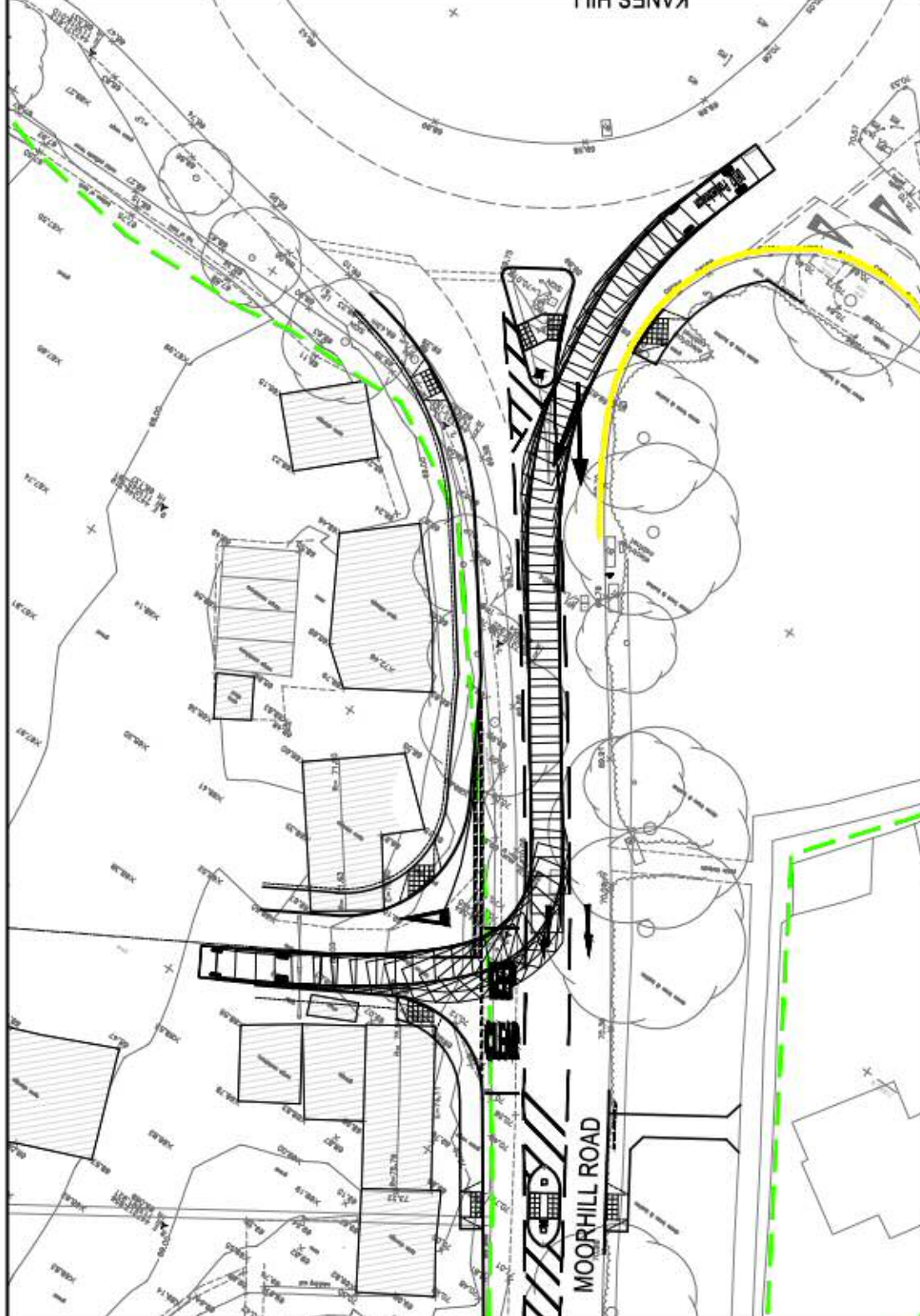
PANTECH COMING FROM ROUNDABOUT, USING TURNING LANE AND GHOST ISLAND TO TURN RIGHT INTO SITE IN FORWARDS GEAR.
