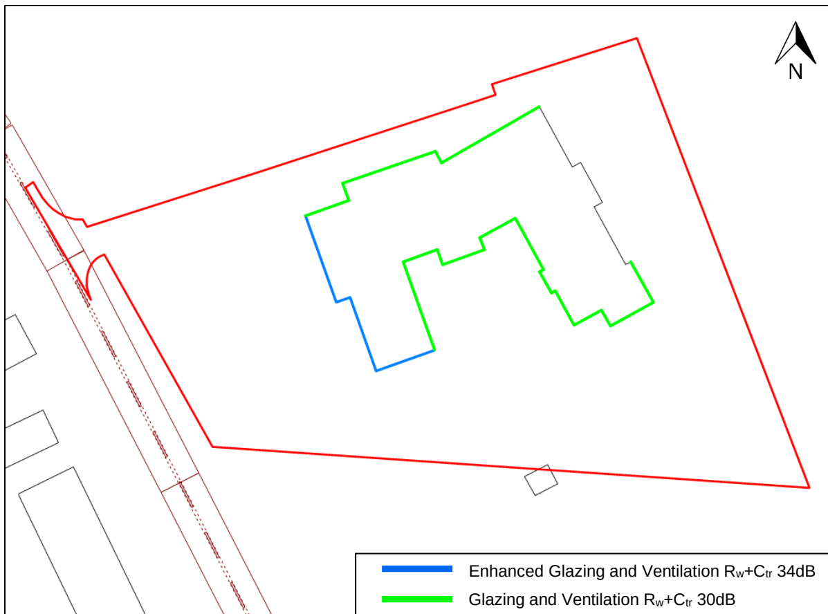
Figure 6.1 Ground Floor Glazing and Ventilation Strategy
