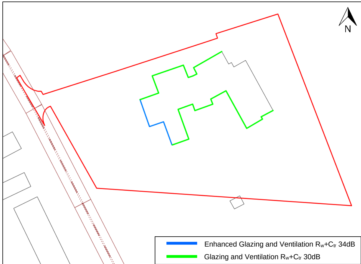
Figure 6.3 Second Floor Glazing and Ventilation Strategy
