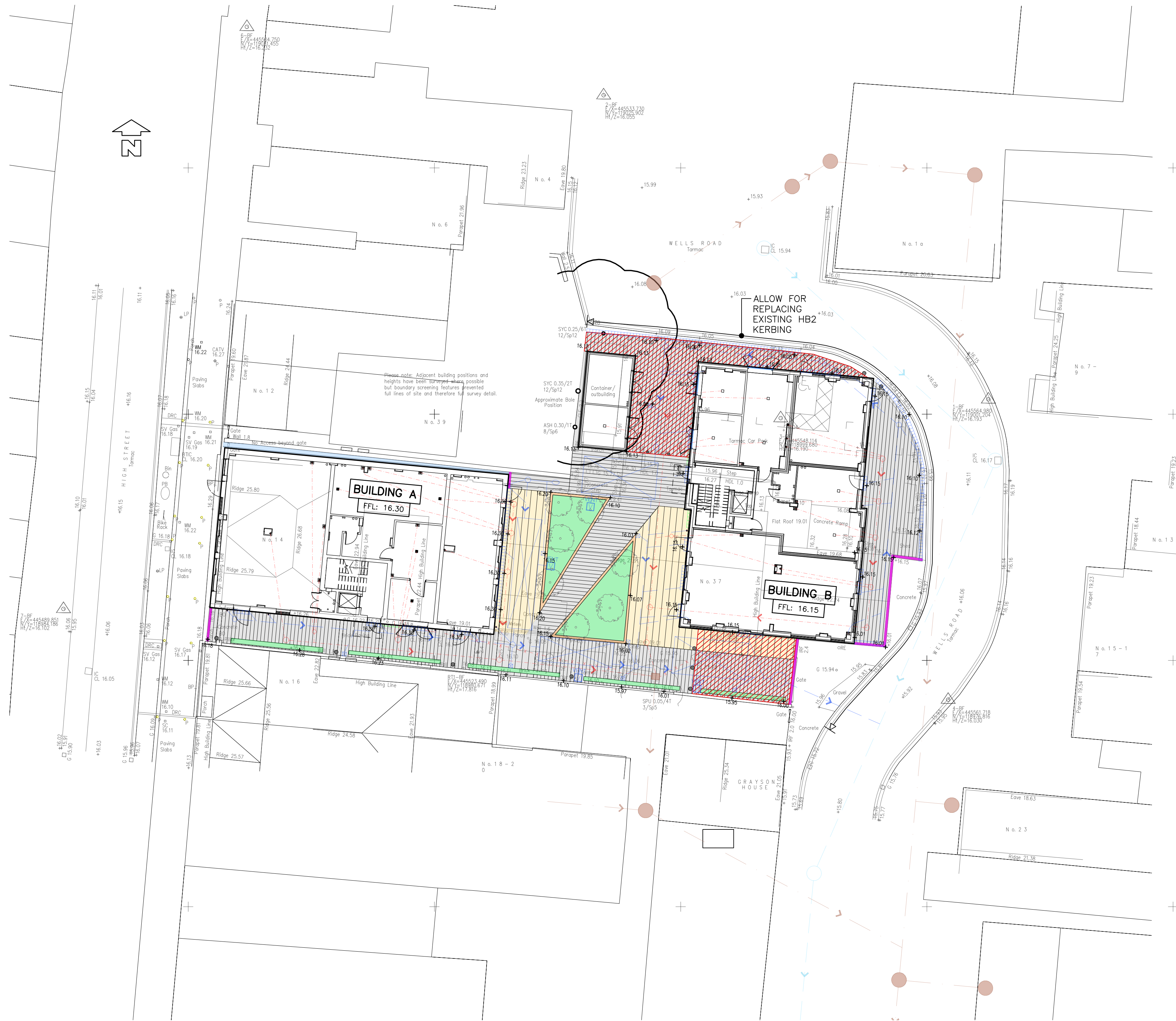
SITE PLAN SHOWING PROPOSED FINISHED EXTERNAL LEVELS (SCALE 1:200 @ A1)
