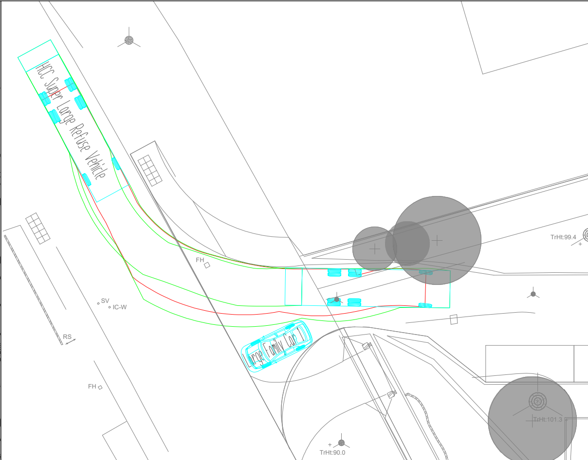
REFUSE VEHICLE AND PRIVATE CAR TWO-WAY ACCESS TRACKING (SCALE: 1:250)
