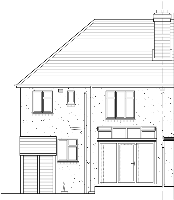
Existing Rear Elevation
