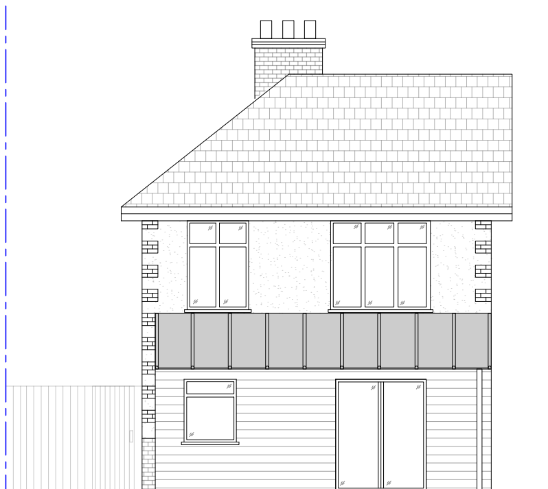
Existing Rear Elevation 1:100 @A3
