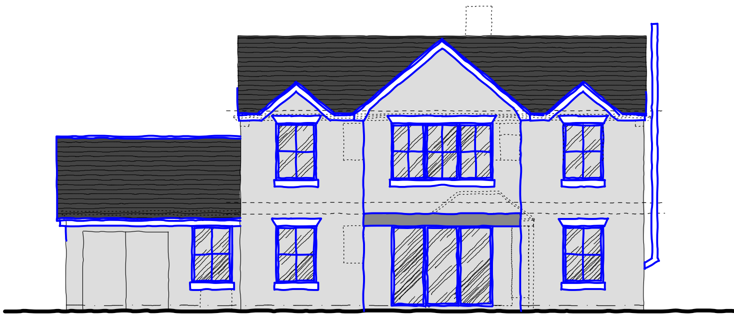
Proposed Front Elevation 1:100
