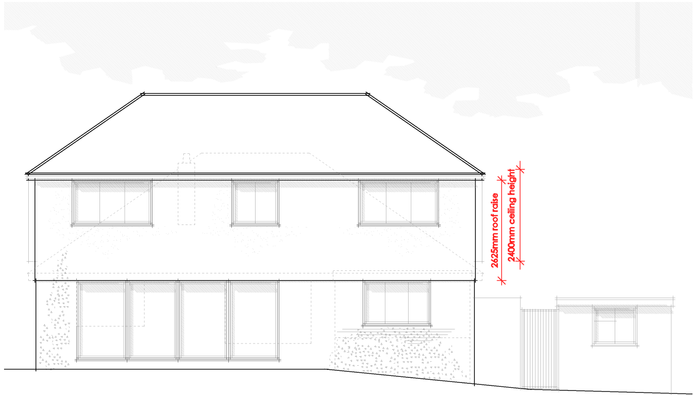
PROPOSED REAR ELEVATION (facing due north west) SCALE 1:100
