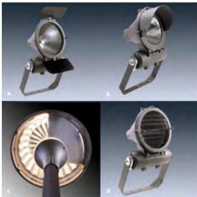
Figure 36. (a) Shield 'barn doors' (b) cowl hood; (c) shield and; (d) external louvre Images from ILP (2011).
