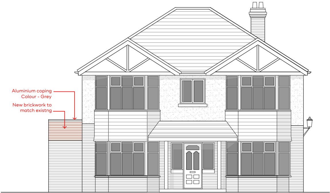
◇ PRINCIPAL ELEVATION (EAST FACING)
