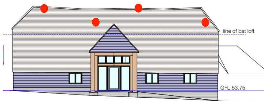
Figure 35. Location of bat tiles on southern facing aspect of building B.
