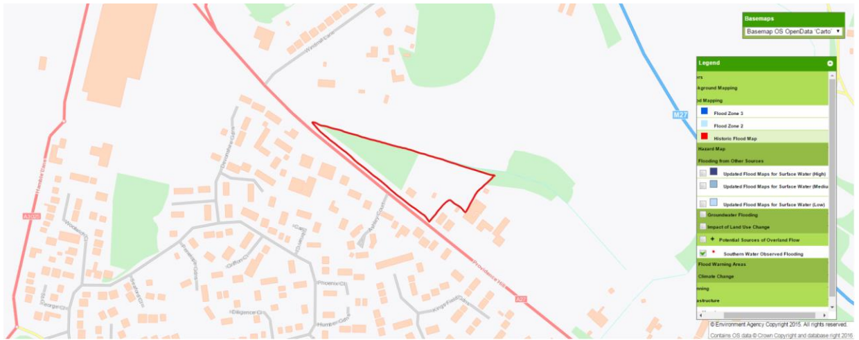
Figure 16: Southern Water Observed Sewer Flooding
