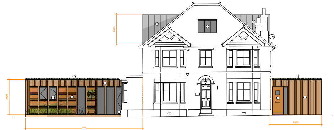
North West Elevation
