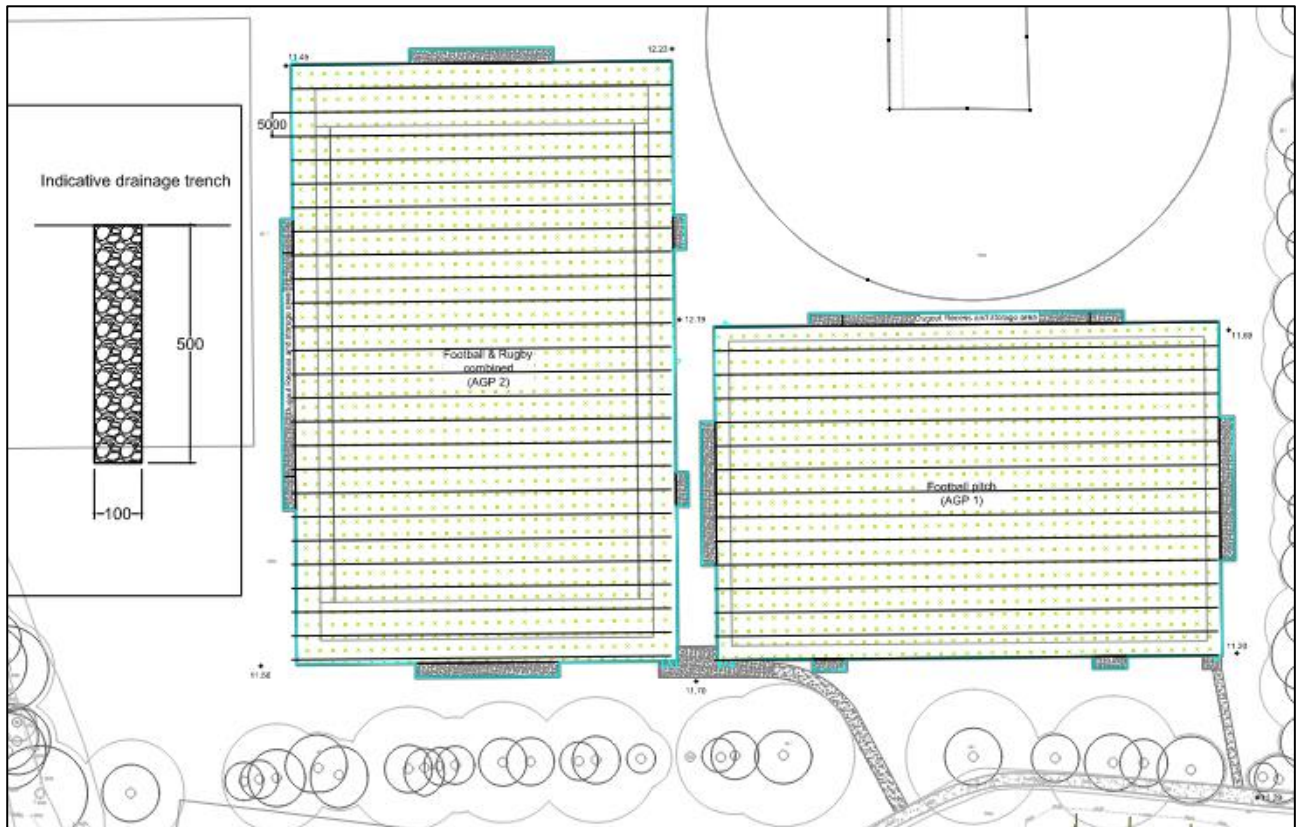
Figure 4 - Indicative pitch drainage layout
