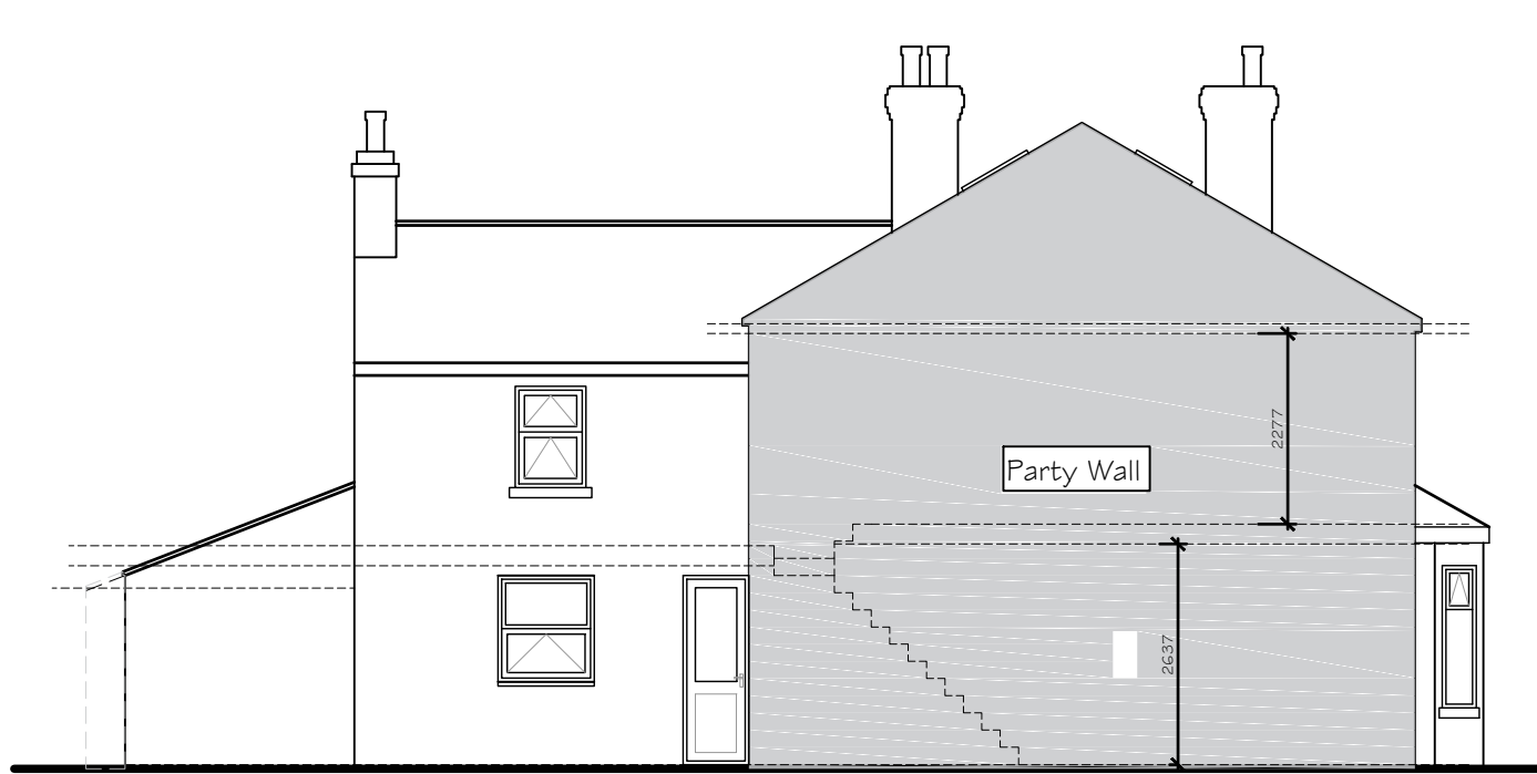
Existing Side Elevation
