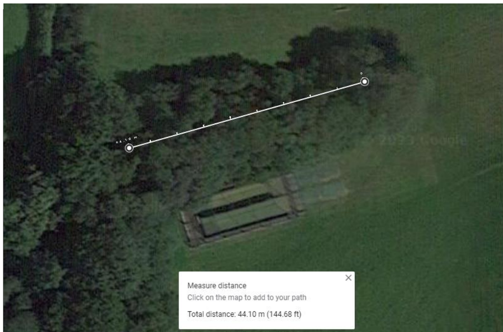
Figure 1: Length of culvert to be extended
