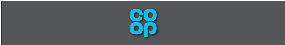
Item 6a 1No Grey folded aluminium fascia panel fixed to the building substrate with suitable fixings. Finished in RAL Grey 7043. Size: 8000mm x 1250mm (approx.) FFL: 3500mm Scale: 1:50
