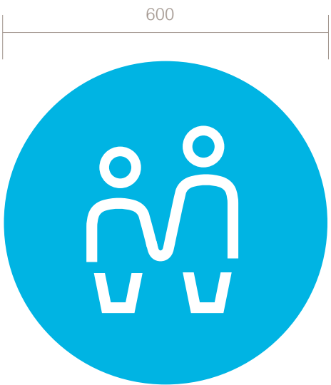
Item 9 1No 3mm ACM with applied vinyl and anti-graffiti laminate. Size: 600x600mm FFL: 1400mm Scale: 1:10
