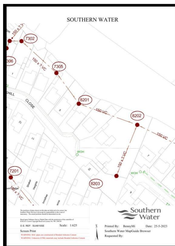
Fig 2: Sewer pipeline location and 'run'.
