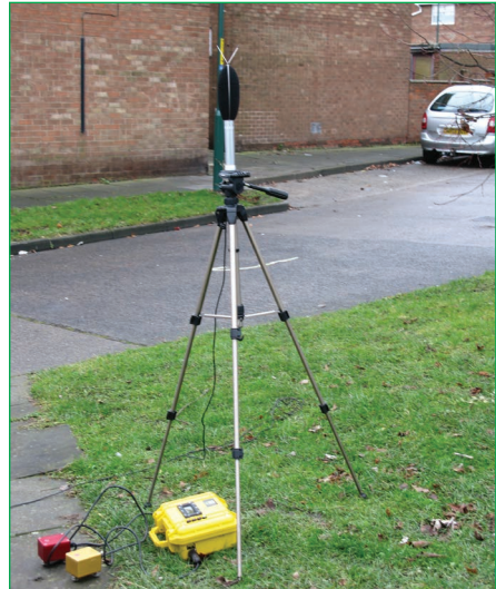
Figure 4.35 Free-field noise monitoring equipment (courtesy Parsons Brinckerhoff)
