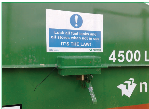
Figure 3.10 Locked fuel tanks (courtesy BAM Nuttall)
