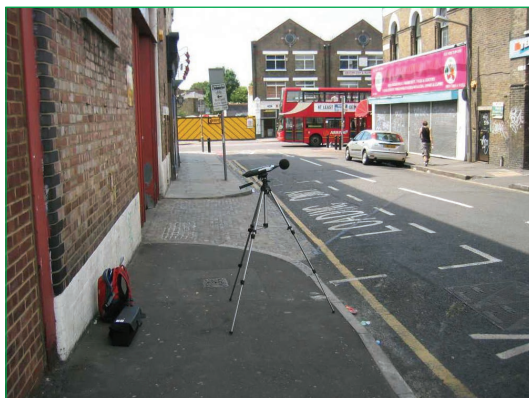
Figure 4.34 Façade noise monitoring equipment (courtesy Arup)
