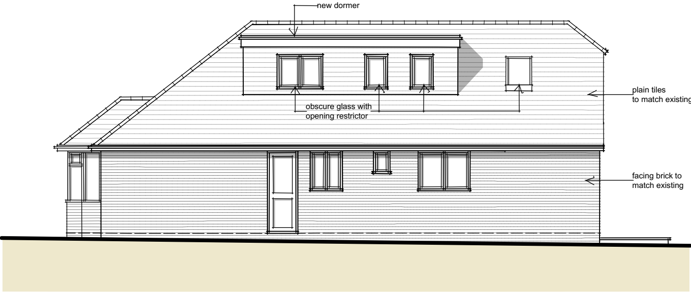
Side (North) Elevation
