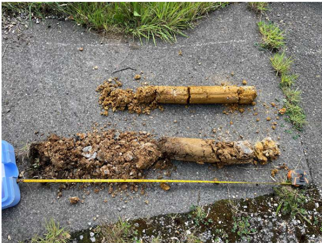
WS03 – encountered ground conditions.
