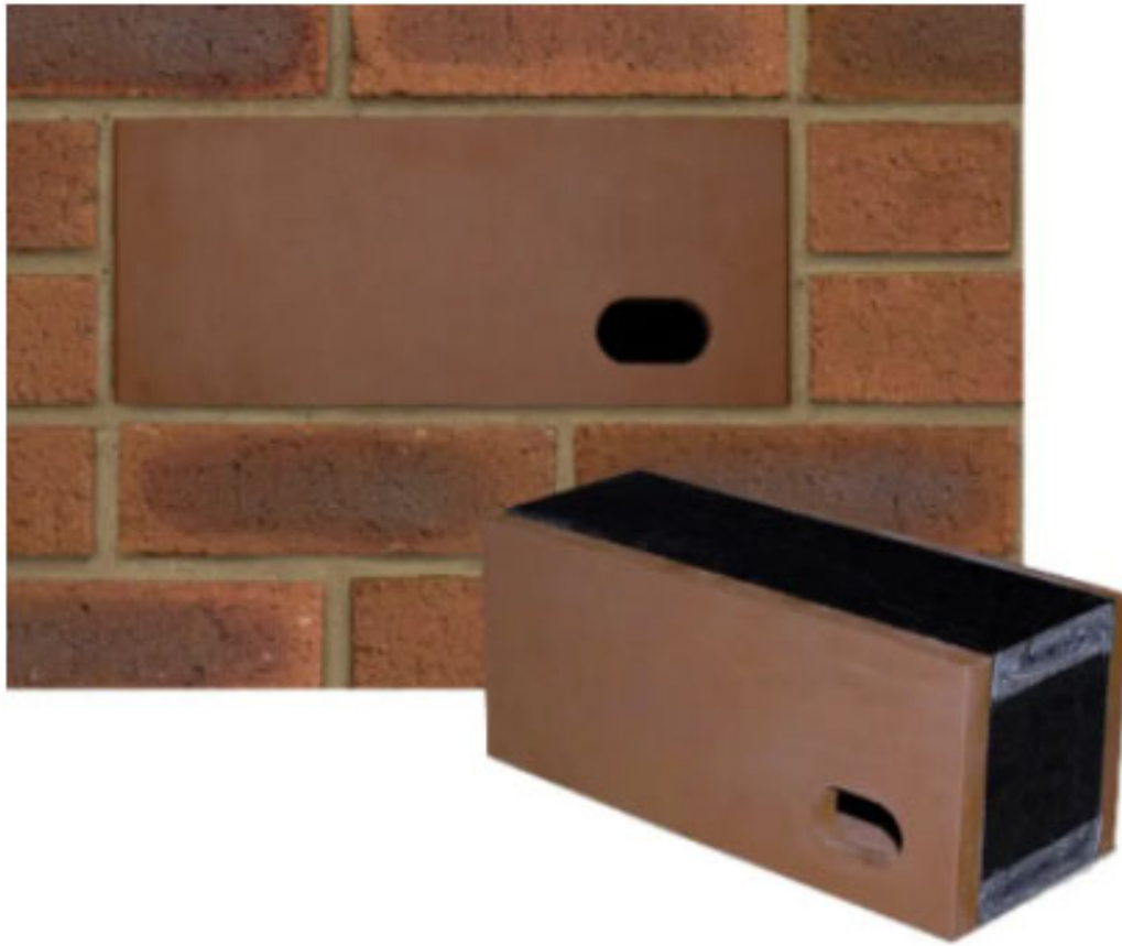
Ibstock Eco-habitat Swift Boxes: • Width 326 x height 140 x depth 140mm; • Weight 4.5kg; • Colour: Buff; • To be integrated within external wall construction
