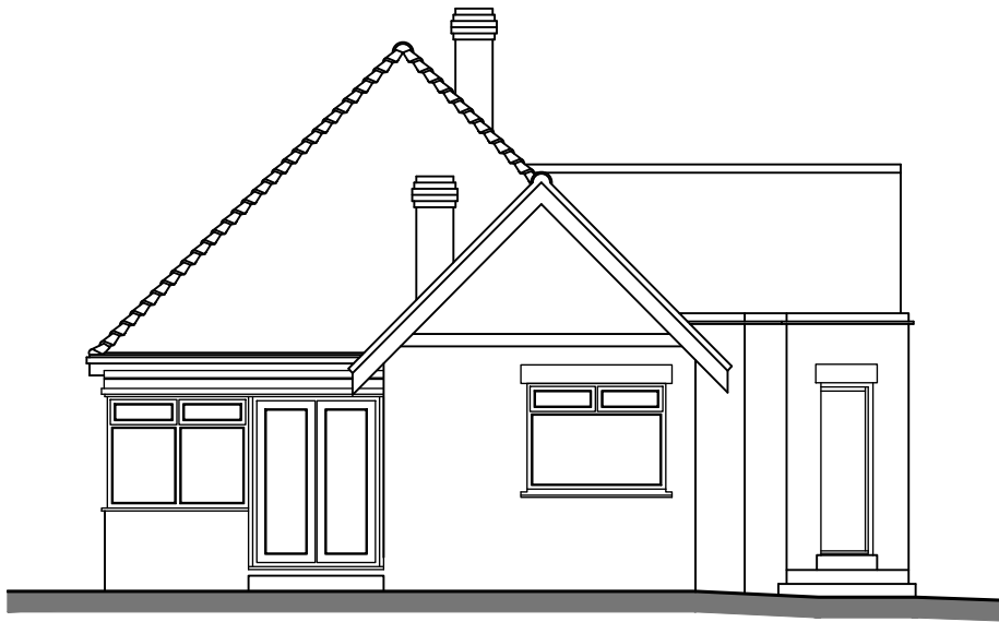
EXISTING SIDE ELEVATION 1:100@A1
