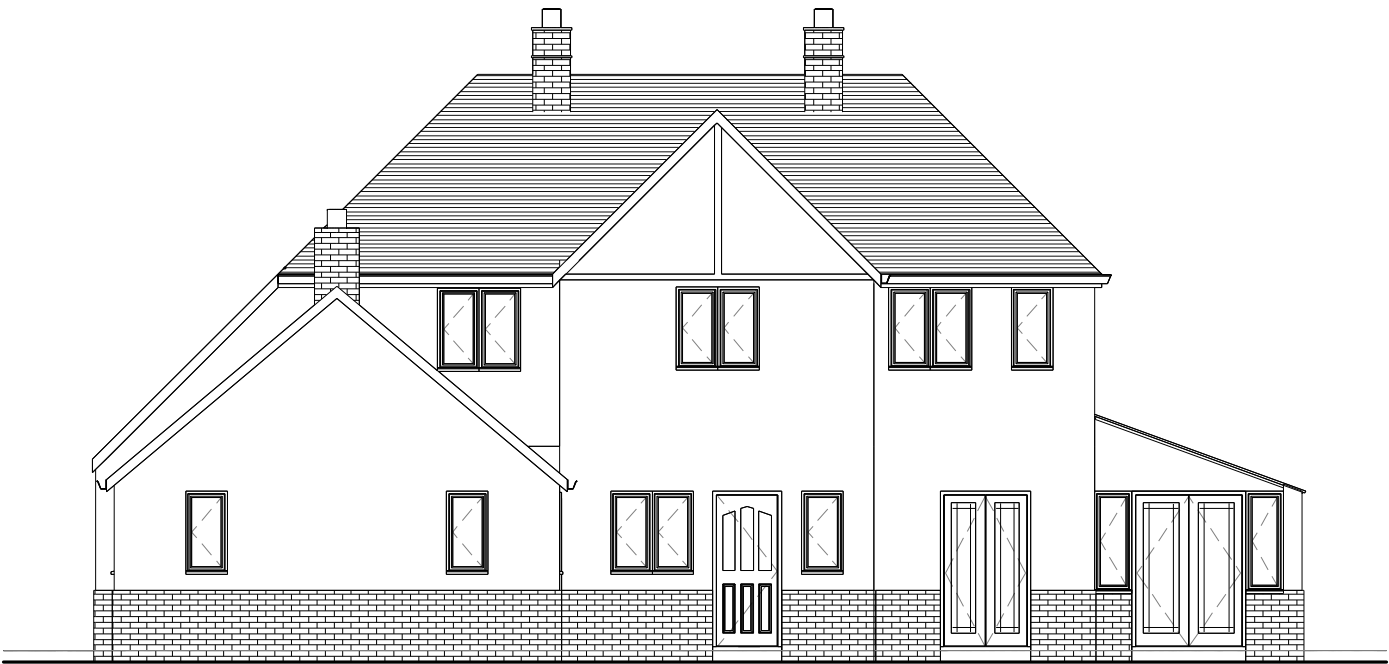
Existing Rear Elevation 1 : 100
