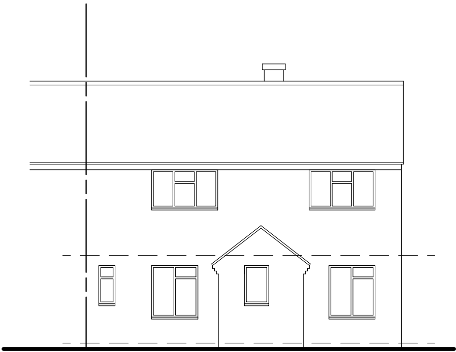
Existing Front Elevation 1:100
