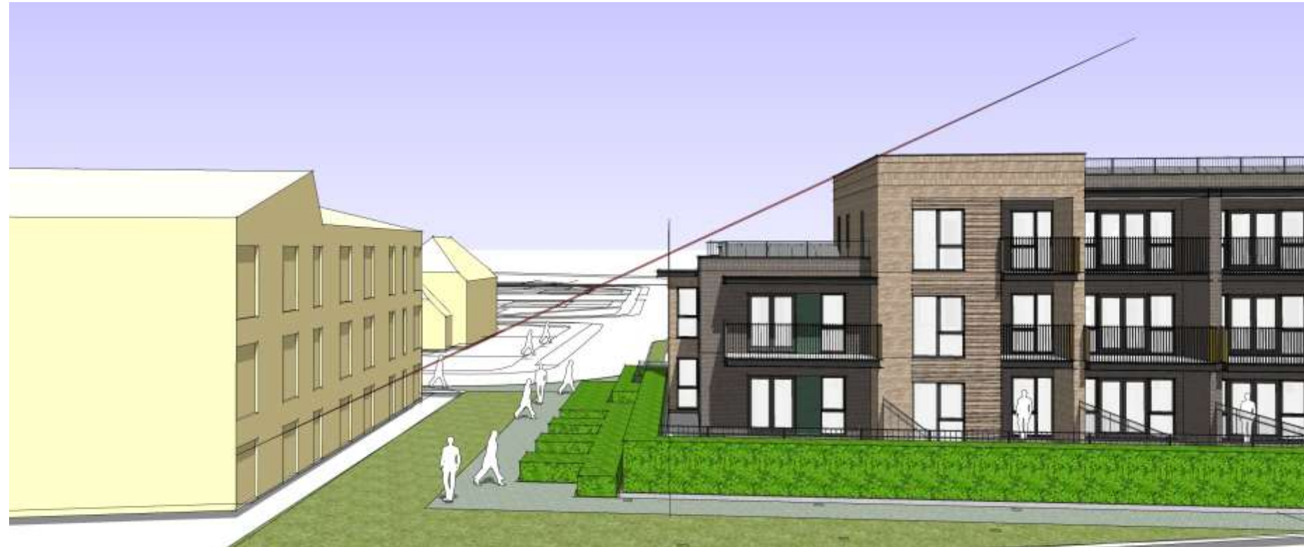
12m minimum setback / 25 degree daylight line for existing flats on Robin Place and proposed apartments on site
