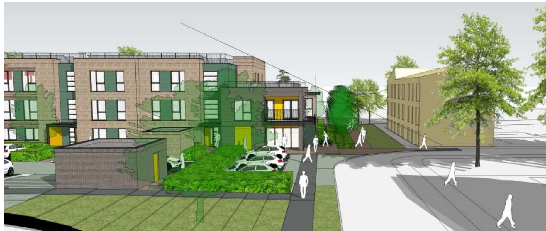
12m minimum setback / 25 degree daylight line for existing flats on Robin Place and proposed apartments on site
