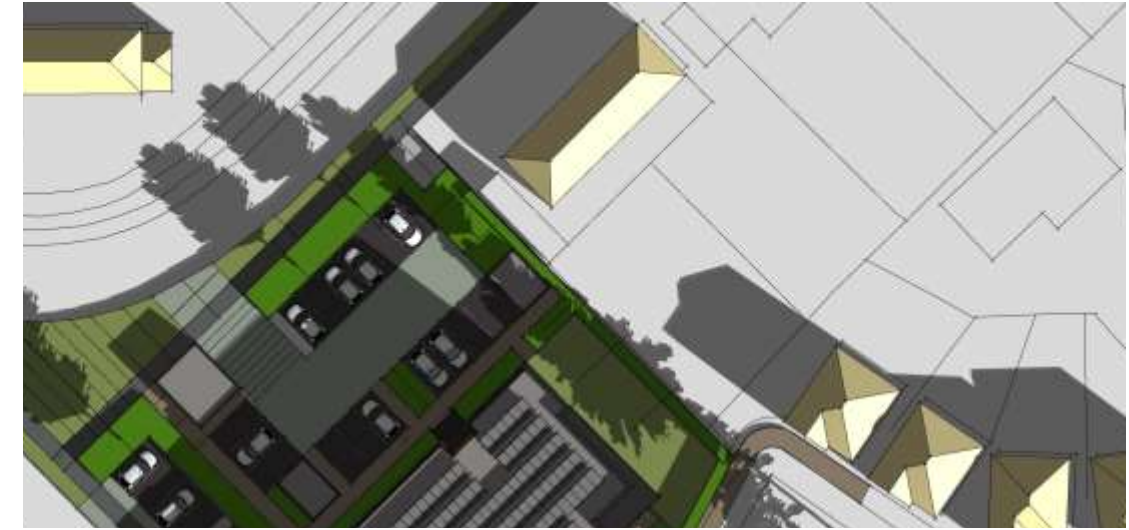
Spring / Autumn Equinox 9am - proposed building shadowing
