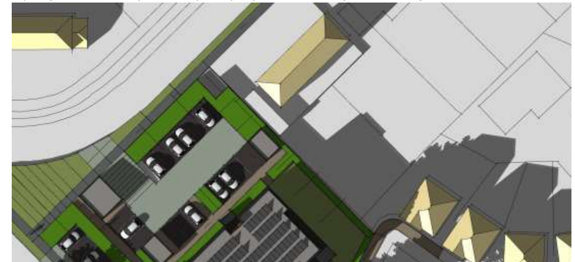
Spring / Autumn Equinox 3pm - proposed building shadowing
