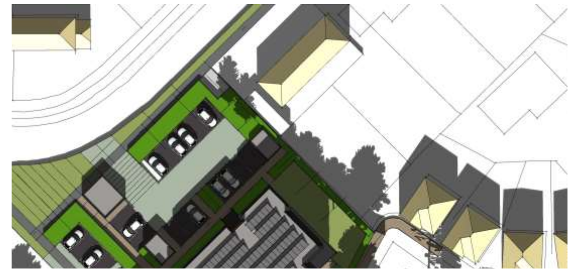
Spring / Autumn Equinox 12pm - proposed building shadowing
