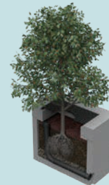
Hydro Biofilter™ Biofiltration System
