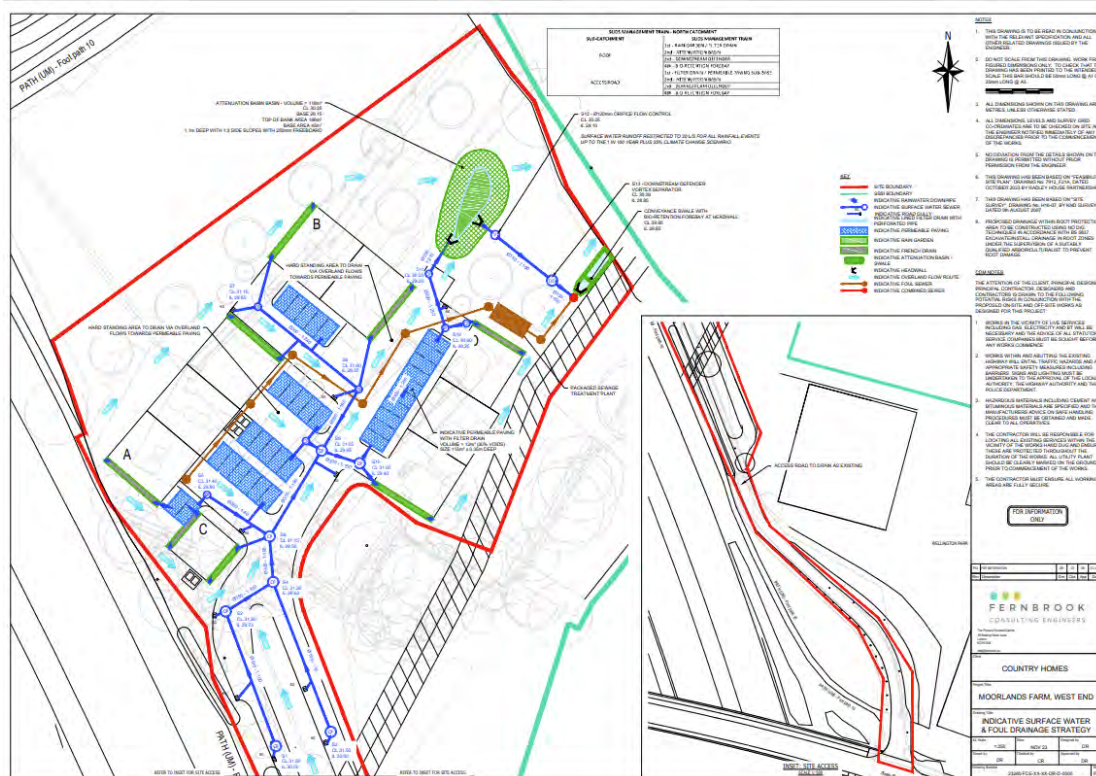
Figure 31. Drainage plan (Fernbrook consulting 2023).
