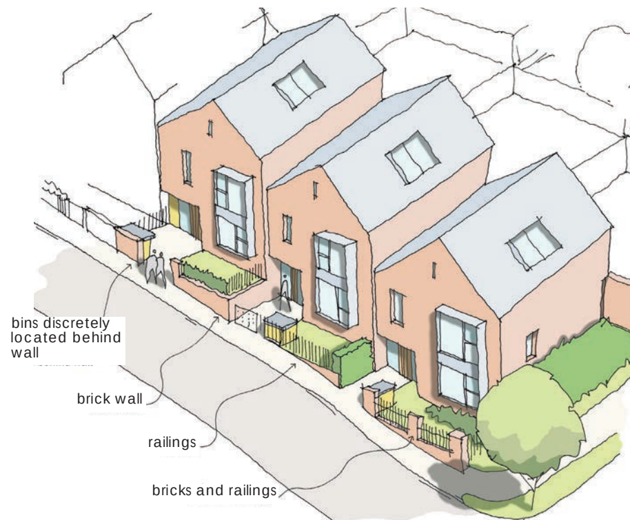
Fig.32: Appropriate boundary structures for front private gardens
