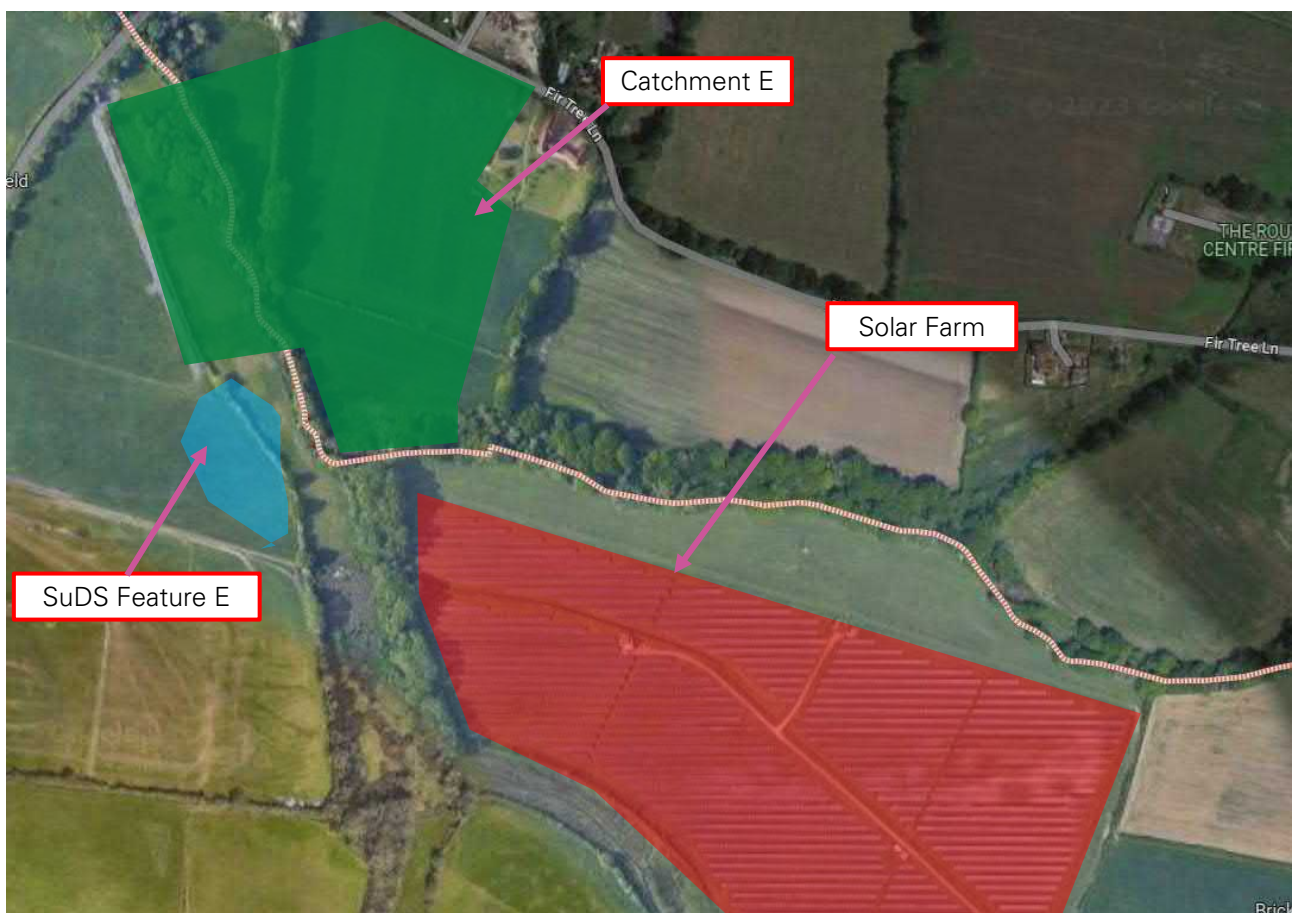
Figure 2: Location of catchment E and its discharge location, Suds Feature E
