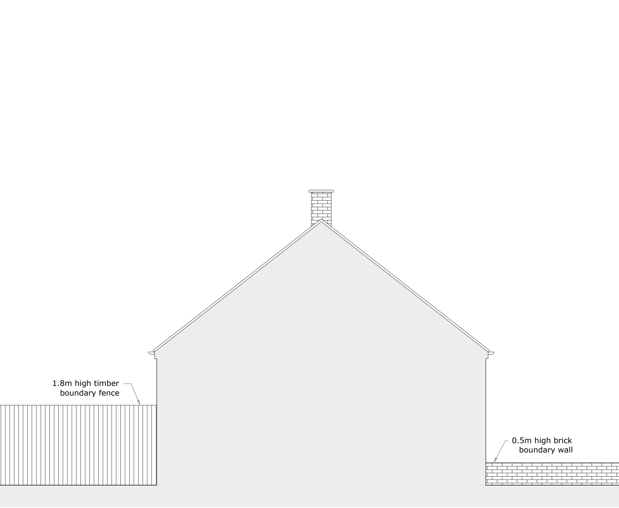
side elevation (south east facing) as existing 1:50
