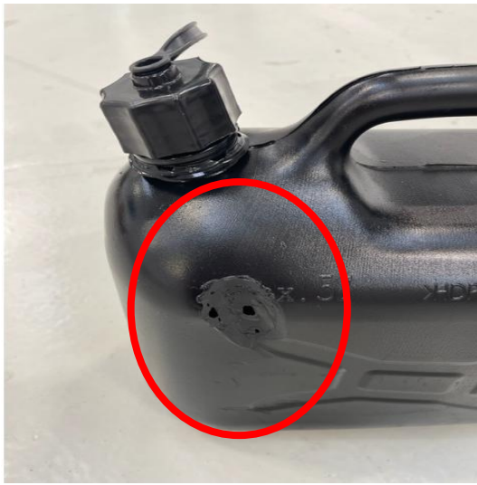
Figure 2 - Damage Caused to Incorrectly Stored Fuel Container
