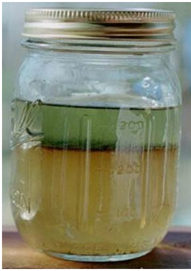
Figure 9 - Example of Microbiological Growth
