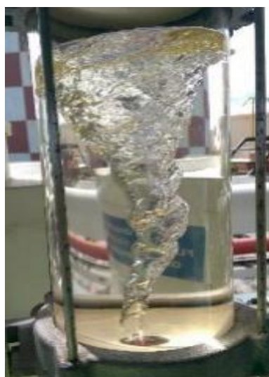
Figure 6 - Example of good vortex created by Visijar Sampler
