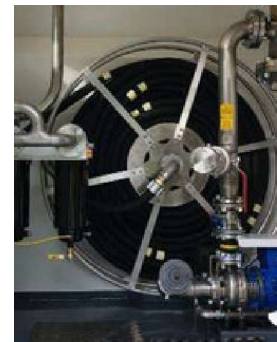
Fuel Proof hydraulic powered hose reel with 30m x 1" Elaflex HD25
