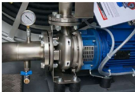
Optional loading pump (Generally a requirement for Avgas tanks, and also Jet A1 in some regions)
