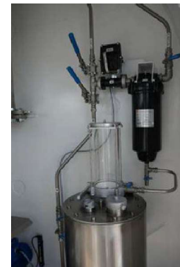
Fuel Proof fuel sampling, inspection and recovery system, with 4L Closed Circuit Sampler
