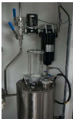
Fuel sampling, inspection & recovery system, with pump and Facet VF-22SB return filter (included)
