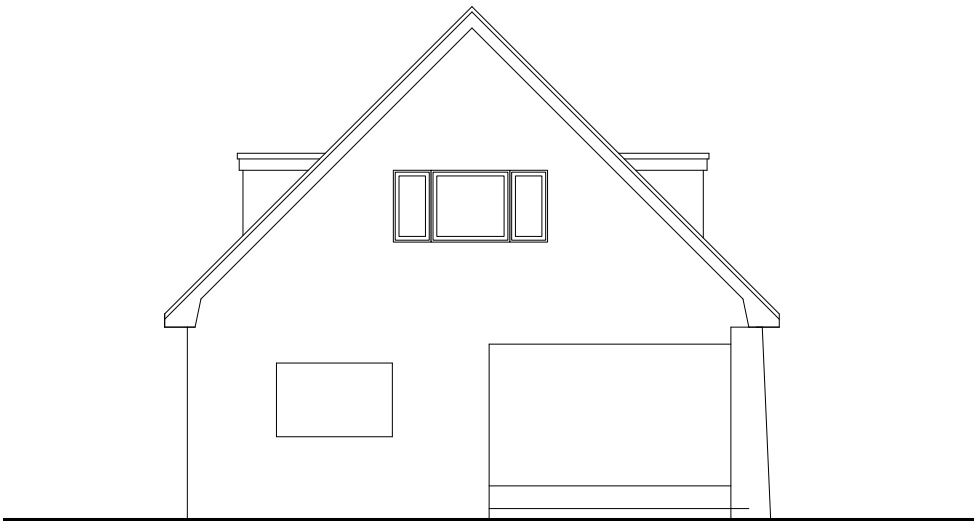
EXISTING FRONT ELEVATION 1:100
