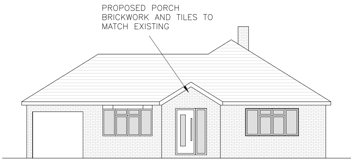
PROPOSED FRONT ELEVATION SCALE 1:100
