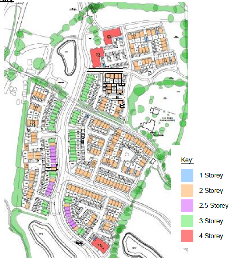
Figure 4 – Quobleigh Breach Storey Heights
