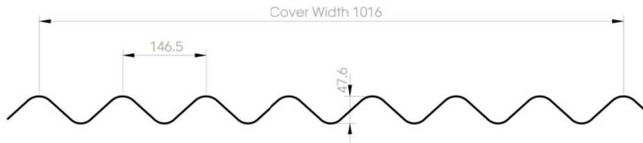
profile of roof sheet
