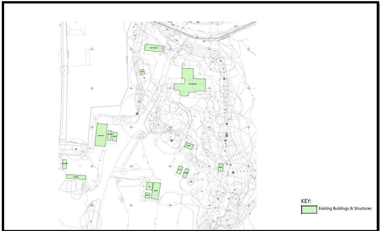
Fig 2: Buildings and structures highlighted for removal.
